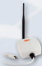
Radio Répéteur: to use in case of obstacles that inhibit radio transmissions. 220V power supply
