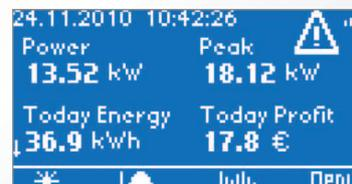
Thanks to the solar irradiance and temperature sensor (accessory) it is possible to check on the display the efficiency of the plant as well as possible alarms in case of performance drop.
